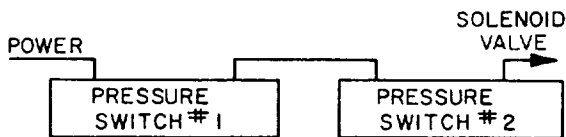
Figure 2-8.—Noncomplex series redundancy. (This type of redundancy guards against inadvertent closing, i.e., closing when not called upon to close.)
